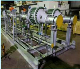
Furnace Cooling System (Steel & Copper)
